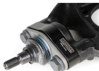
Figure 1- The roll centre adjuster unit without washer
