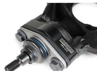
Figure 2- The roll centre adjuster unit with washer
